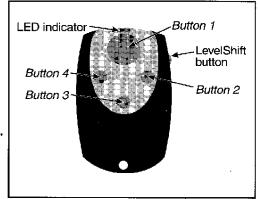
LevelShift button twice, then press button 2. While you transmit, you'll notice that the LED blinks three times, pauses, blinks three times, etc.: this indicates level 3.
