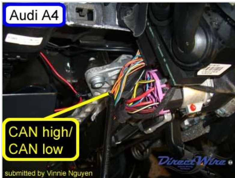
Wiring Photo and Notes: Can Bus High
