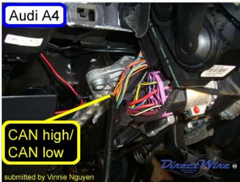
Wiring Photo and Notes: Can Bus High
