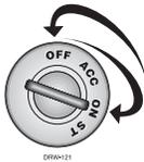
2. **Ignition.** Turn the ignition on, then back off. (The heavy gauge PINK wire of the relay satellite must be connected.)
