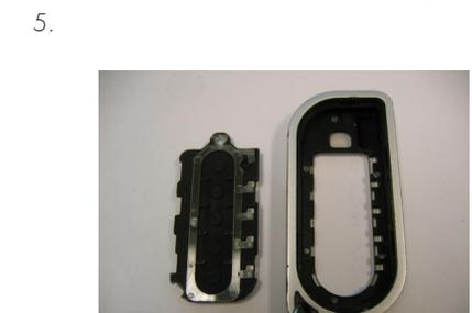
6. Insert Keypad assembly into Front Housing and Outer Bezel.
