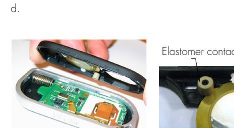
1. Turn the remote control over and remove the battery door.
