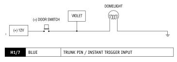
This input responds to a negative input with an instant trigger.
