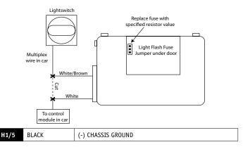
We recommend that you do not use a factory ground. Ground all your components to the same point in the vehicle, (preferably the kick panel). Scrape away any paint and use a factory bolt or make your own ground with a self-tapping screw and a star washer.
