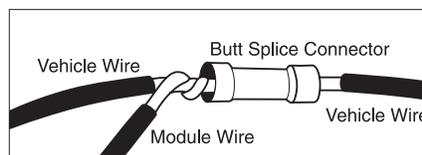
3. Insert the twisted pair of wires into one end of the butt connector and crimp securely.
