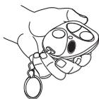
4. Program the feature: While HOLDING the Valet/program switch, you can toggle the feature on and off using your factory remote transmitter. Pressing the button that locks the doors will select the one chirp or default setting. Pressing the button that unlocks the doors, will select the two chirp setting. NOTE: The Valet pulse count feature (9) has five possible settings. Pressing the transmitter unlock button will toggle through all the two-chirp settings.
