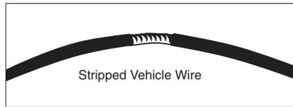
2. Twist the security module's wire around the bare section of the vehicle's wire.
