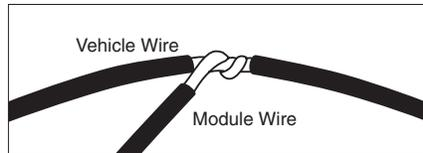
3. Solder the bare connection thoroughly using rosin core solder.
