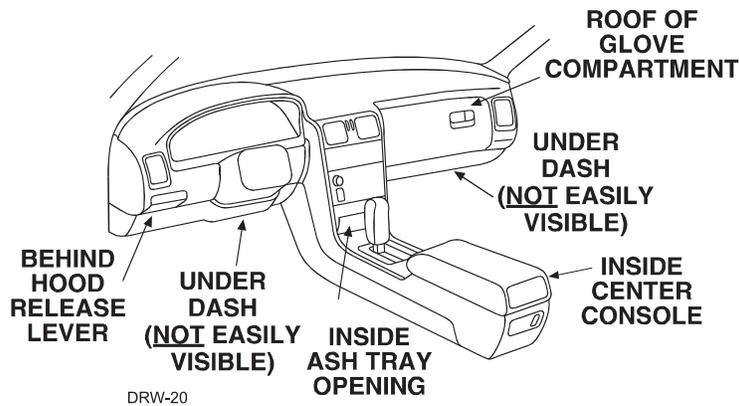
**IMPORTANT!** When the vehicle is delivered, please show the user where the switch is located and how to disarm the system with it.
