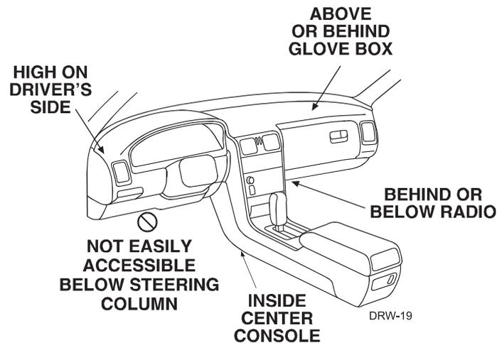
Some good control module locations: above the glove box, inside the center console, above the under-dash fuse box, above the radio, etc.
