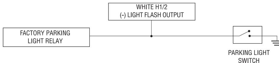
**NOTE:** For parking light circuits that draw 10 amps or more, the internal jumper must be switched to a (-) light flash output. (See the *Internal Programming Jumper* section of this guide.) **P/N 8617** or a standard automotive SPDT relay must be used on the H1/2 light flash output harness wire.
