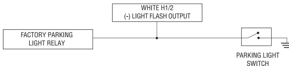
**NOTE:** For parking light circuits that draw 10 amps or more, the internal jumper must be switched to a (-) light flash output. (See the *Internal Programming Jumper* section of this guide.) **P/N 8617** or a standard automotive SPDT relay must be used on the H1/2 light flash output harness wire.
