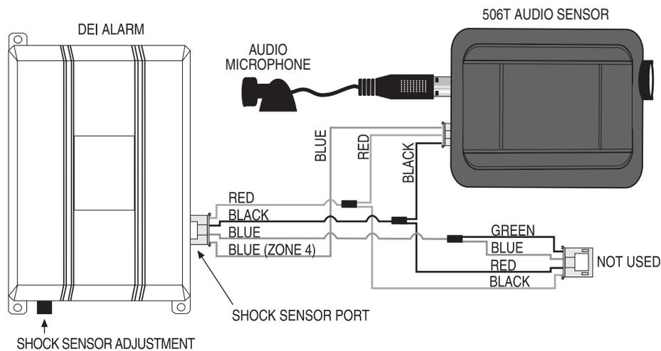
**Adding a 506T to a security systems without a shock sensor input or to a DEI system with an external shock sensor that does NOT report separate zones on the shock sensor port**
