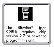
Bitwriters with a date code of 6a or older require an IC upgrade (p/n 998M). Some bitwriters with a date code of 6B do not require the IC upgrade, refer to tech tip # 1112 for more information.
