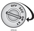
2. **Turn the ignition on.** (The YELLOW wire, H1/9 must be connected.)
