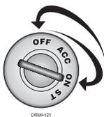
2. **Ignition.** Turn the ignition on, then back off: (The H1/4 YELLOW wire must be connected.)
