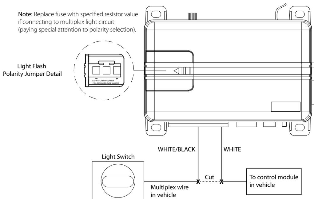
*[Vehicle specific optional connection both configurations]*
