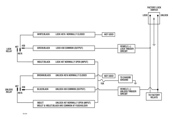
Wiring Diagram C, Directly-Wired Reversing-Polarity Switch Circuits
