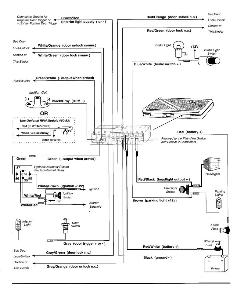
Wiring Description for the 18-Pin Connector
