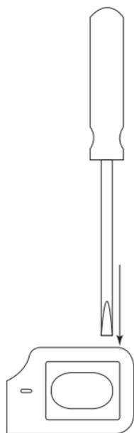
1. Using a small slotted screwdriver, insert into slot located on the side of the unit as shown and carefully pry the front of the unit up, working your way around the edge until the front is completely separated from the housing.
