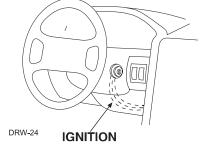
5. Now turn the key to the start position. The meter display should stay steady, not dropping by more than a few tenths of a volt. If it drops close to or all the way to zero, go back to Step 3. If it stays steady at (+)12V, you have found an ignition wire.
