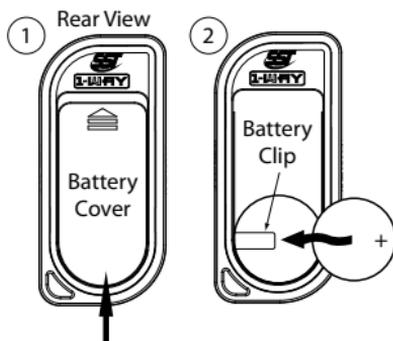
1. Slide the battery cover up by applying equal pressure at its top and bottom (the arrow on the cover indicates the direction), remove the cover from the remote control housing.
