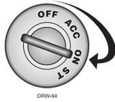
To disarm the security system, turn the ignition to the ON position. Press and release the Valet switch within 10 seconds. The status LED will stop flashing and the vehicle should start. If the vehicle does not start, you may have waited too long; turn the ignition off and repeat the process.
