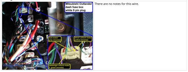
Wiring Photo and Notes: Passenger Unlock Motor
