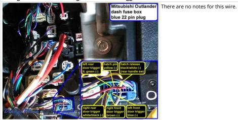
Wiring Photo and Notes: Left Rear Door Trigger
