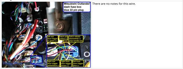
Wiring Photo and Notes: Trunk/Hatch Release
