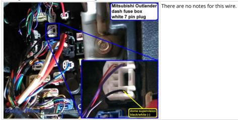
Wiring Photo and Notes: Trunk/Hatch Pin
