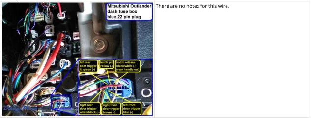
Wiring Photo and Notes: Trunk Release Motor
