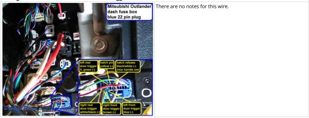
Wiring Photo and Notes: Right Rear Door Trigger
