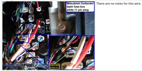
Wiring Photo and Notes: Horn Trigger
