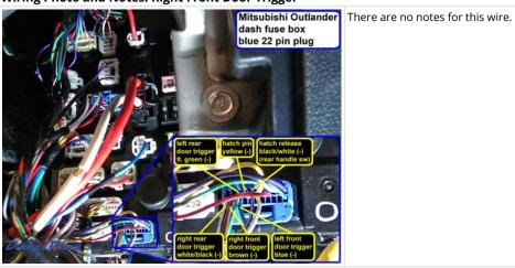
Wiring Photo and Notes: Left Rear Door Trigger
