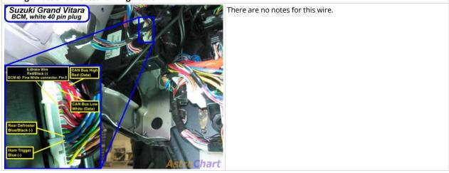
Wiring Photo and Notes: Horn Trigger
