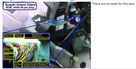
Wiring Photo and Notes: Right Front Door Trigger
