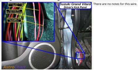
Wiring Photo and Notes: Left Front Door Trigger
