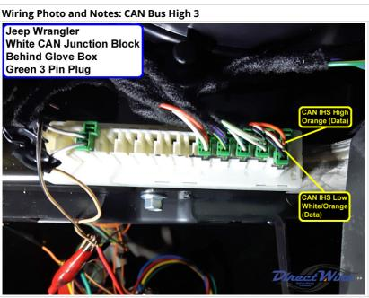
Can also use violet/white at the Security Gateway Module on back of driver dash speaker pod, black 8 pin plug, pin 3.
