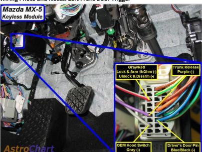
On models with keyless entry, it is also blue/black (-) at the Keyless Control Module above driver kick, gray 27 pin plug, pin 16.
