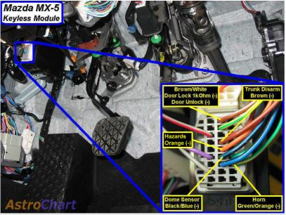
On models with keyless entry, it is also black/blue (-) at the Keyless Control Module above driver kick, gray 27 pin plug, pin 15.
