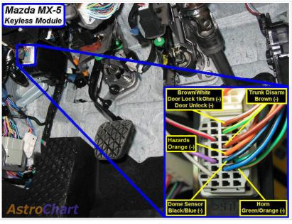
On models with keyless entry, it is also orange (-) at the Keyless Control Module above driver kick, gray 27 pin plug, pin 14.
