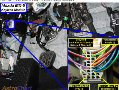
On models with keyless entry, it is also purple (-) at the Keyless Control Module above driver kick, gray 27 pin plug, pin 6.
