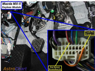
On models with keyless entry, it is also brown/red (+) at the Keyless Control Module above driver kick, white 30 pin plug, pin 25.
