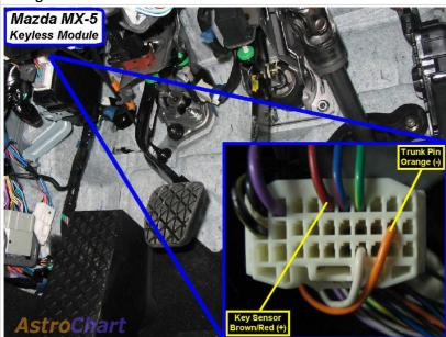
On models with keyless entry, it is also orange (-) at the Keyless Control Module above driver kick, white 30 pin plug, pin 19.
