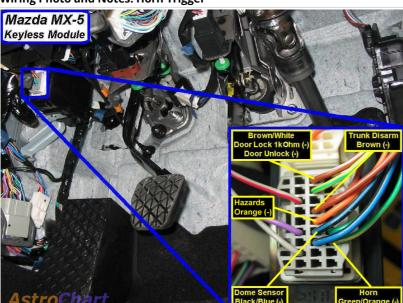
On models with keyless entry, it is also green/orange (-) at the Keyless Control Module above driver kick, gray 27 pin plug, pin 25.
