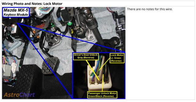
Wiring Photo and Notes: Driver Unlock Motor
