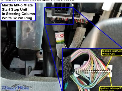
Do this to enable OEM remote during remote start runtime.
