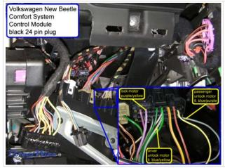
Wiring Photo and Notes: Driver Unlock Motor
