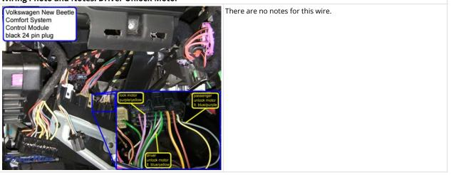
Wiring Photo and Notes: Passenger Unlock Motor
