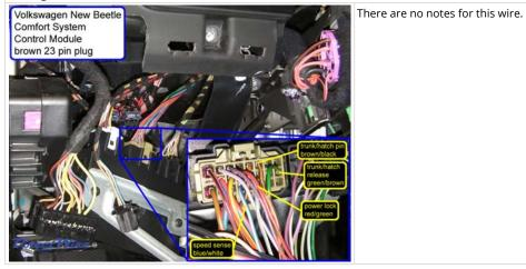
Wiring Photo and Notes: Trunk Release Motor
