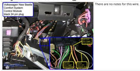
Wiring Photo and Notes: Right Front Door Trigger
