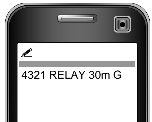
Example: The relay will be switched for 30 minutes at GPS alarm activation
