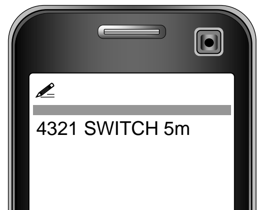
Example: Switch the relay for 5 minutes and after this time period elapses automatically return the relay to its unswitched state
