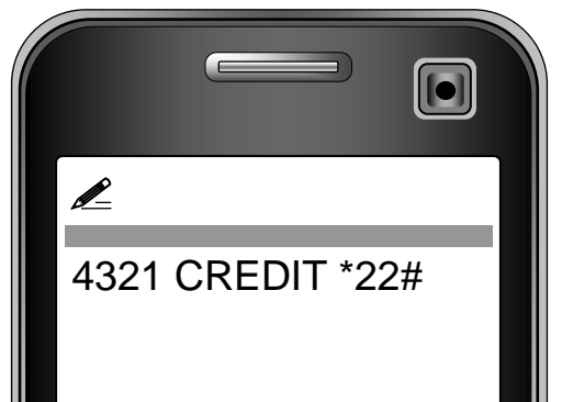
Example: Command for getting info about current credit in a pay as you go SIM card (Vodafone CZ) used in the GPS locator.
