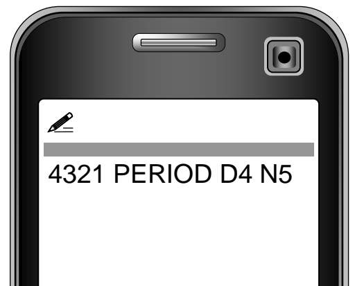
Example: The SMS will be sent after each 4 kilometers covered after GPS alarm activation. It is 5 alarm SMS in total within one activated GPS alarm.
