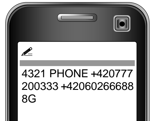
Example: Two authorized phone numbers are entered. To the number +42060266688 will be the alert SMS sent only at GPS alarm activation.
