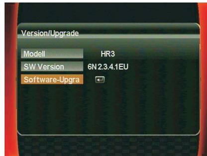
Shows the current software version. A software upgrade can be done by the 4-PIN jack on the bottom plate.
