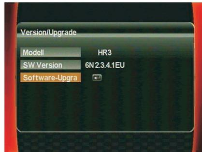
Shows the current software version. A software upgrade can be done by USB.
